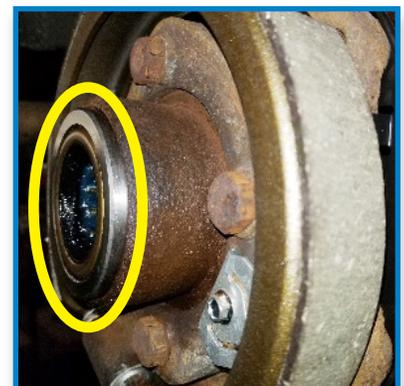
Repair Bearing Extending from Axle Housing
