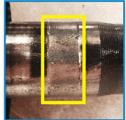
Normal Axle Shaft Wear from OE Bearing Rollers
