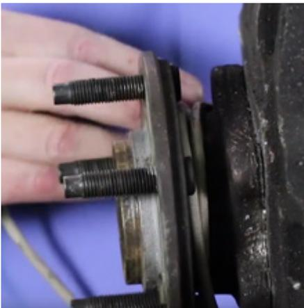
**Mounting flange fused to steering knuckle**
