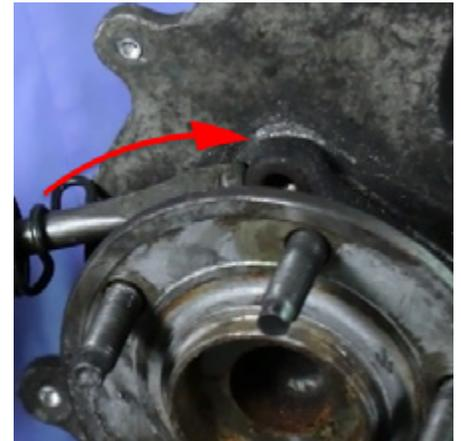
**Use air hammer to rotate flange and break it free**
