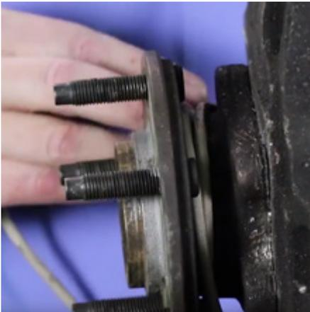
**Mounting flange fused to steering knuckle**
