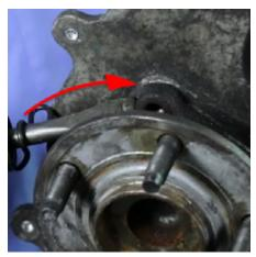
Use air hammer to rotate flange and break it free
